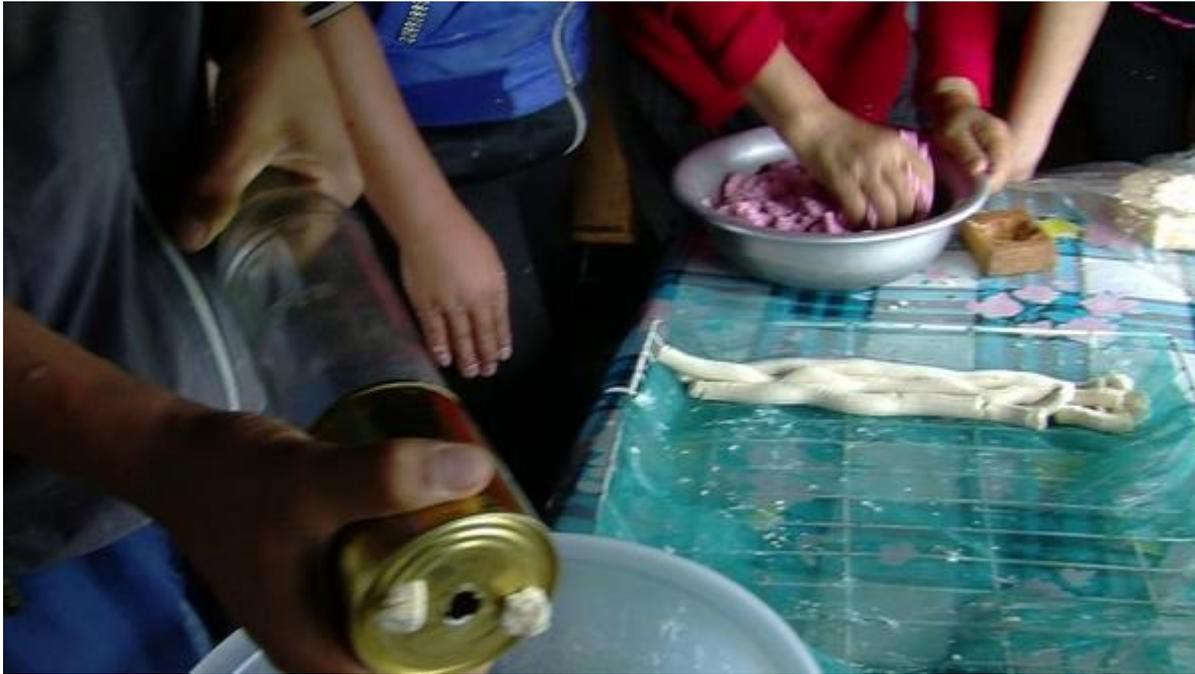
Figure 255: Uganbayar removes the bottle plunger from the extruder.
