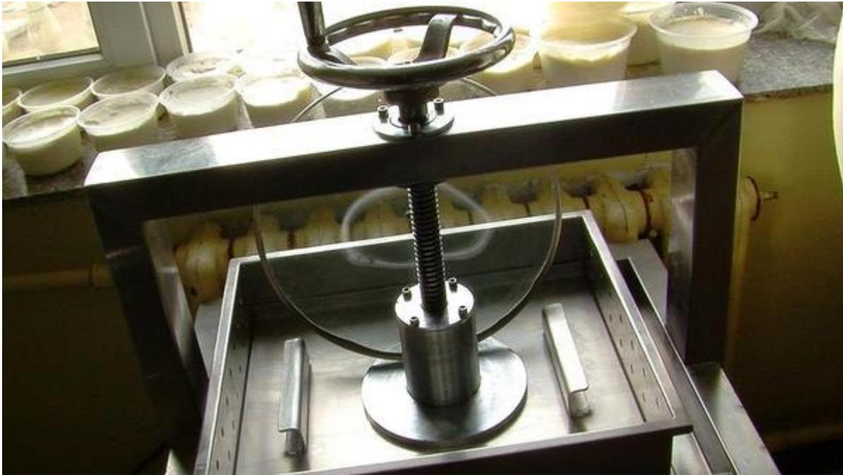
Figure 352: Mechanical press used in making aaruul.
