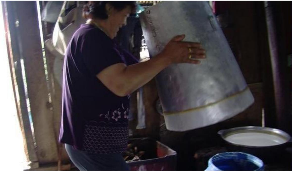
Figure 263: Dolgorsüren assembles her pot still. First she takes her bürkheer, a tapered cylinder fashioned of sheet aluminum, which will serve as the distillation column in the still.
