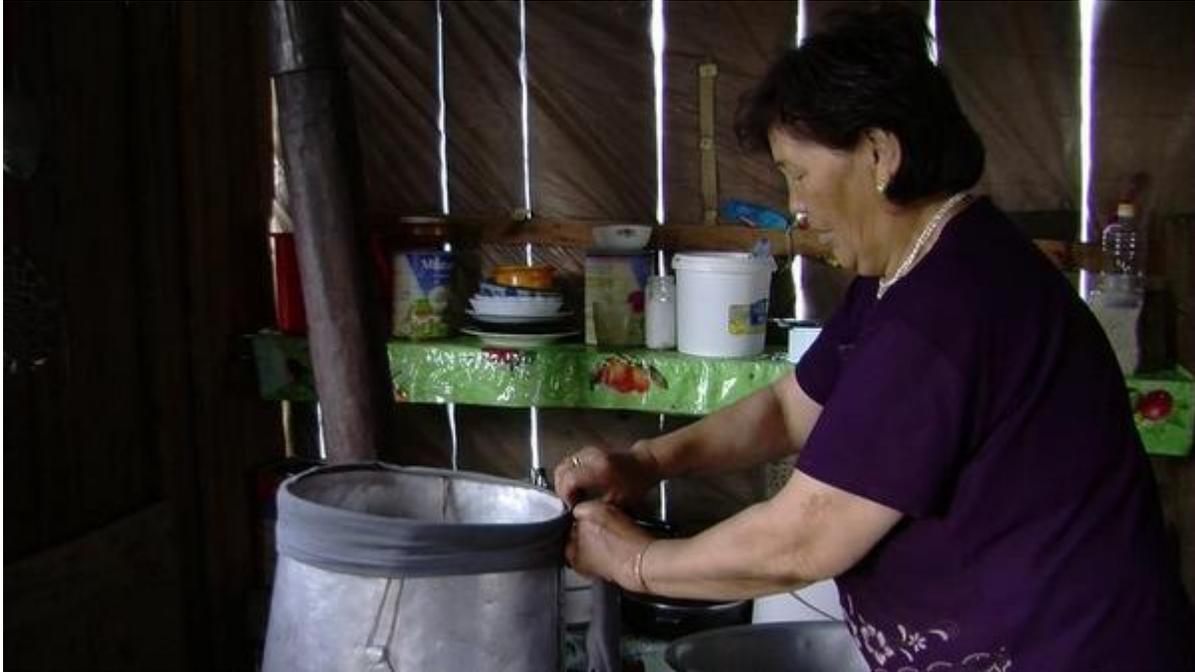
Figure 267: Dolgorsüren wraps a cotton band around the top of the distillation column, to serve as an insulating collar.
