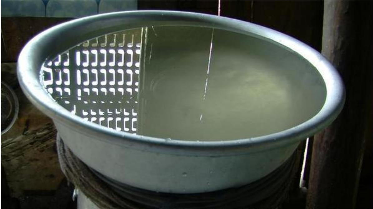
Figure 283: Water inside the top basin. The alcohol vapour will condense quickly on contact with the cold bottom surface of the basin.
