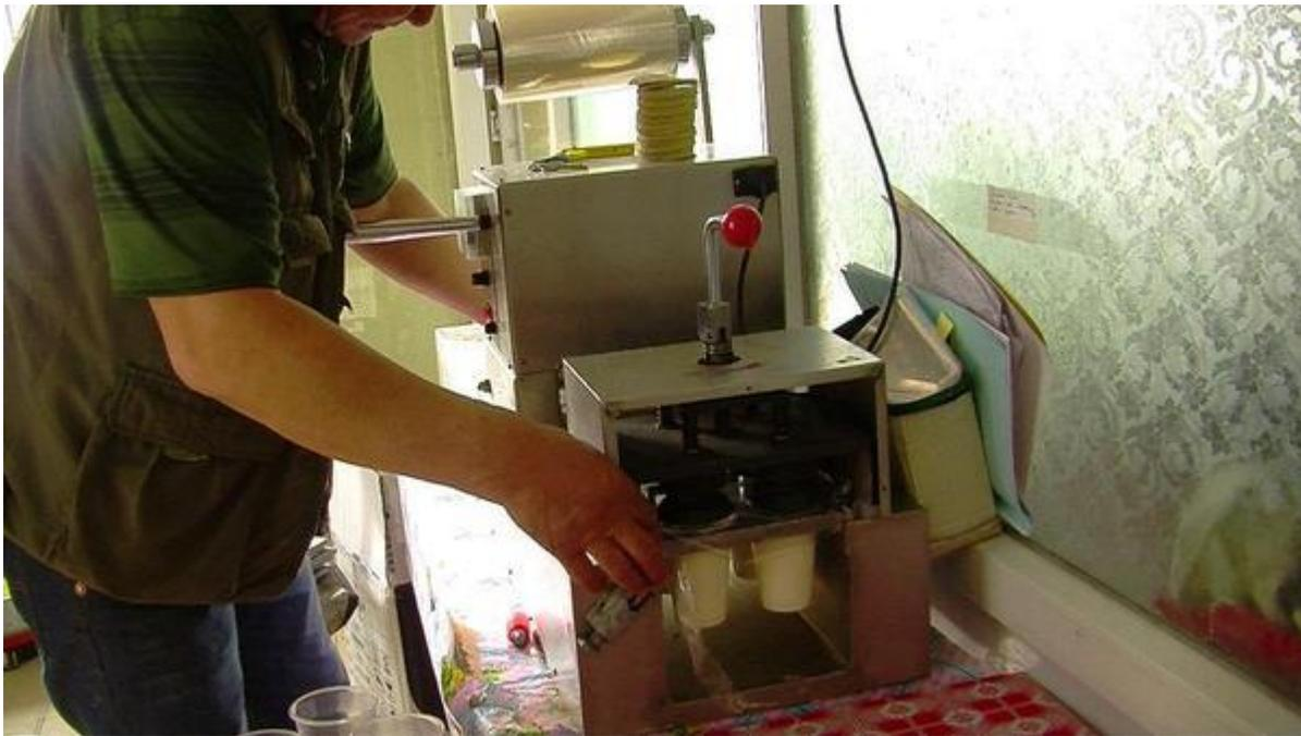
Figure 364: Delgersaikhan feeds the four cups into the sealing machine. Plastic sealing wrap feeds into the machine from a roll at the top, and is adhered to the tops of the cups then cut with a manual crank.
