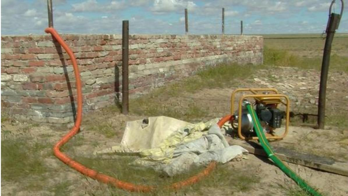
Figure 335: The water pump. Delgersaikhan uses a gasoline pump to draw water from the open reservoir, which then feeds a sprinkler system to irrigate the corn crop.
